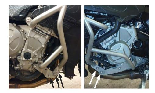
(2) Tighten all M8 bolts on front low brackets and cross tube to 15 N-m.
