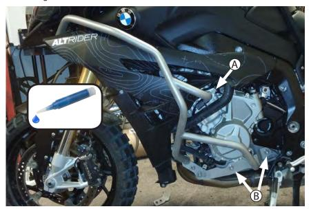
Attach the left side bars to the bike. Position with cross tube under nose, install one M8 x 25 stainless socket cap screw with washer to threaded hole in frame (A). Attach low bracket to threaded holes in bike with two M10 x 20 socket cap screws with washers(B). Leave loose for now. Apply medium strength thread locker to each screw.
