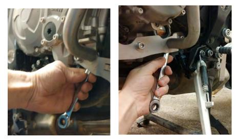
(2) Use 13mm open-end wrench and tighten the M8 hex cap screws from behind the brackets on right and left side.
