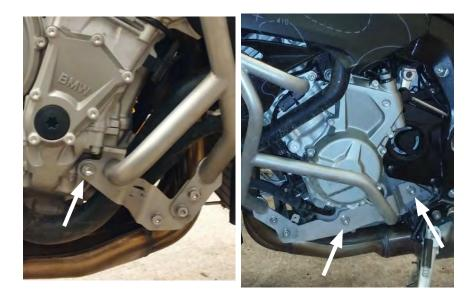
18 Tighten (3) M10 lower engine bracket screws to 25 N-m.
