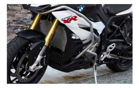
Reinstall lower fairing. Right side torx screw attaches to threaded hole in AltRider bracket. Otherwise installation is reverse of removal.
