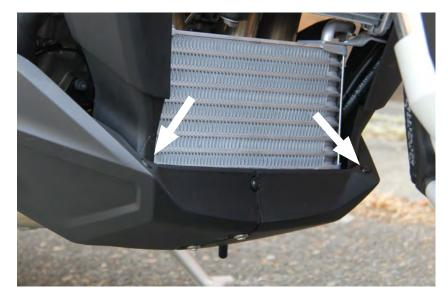
Remove plastic lower fairing. Start by detaching the small plastic rivet at each front corner. Push the small central pin inward. Caution! It will detach and spit out on the inside of the fairing, watch where it goes! Then pull the head of the plastic rivet outwards. Save these parts for re-assembly.
