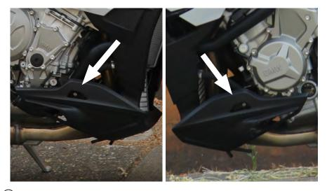
(3) Use a T25 torx bit and remove the two screws (one right side, one left) that attach the lower fairing. Save these for reinstallation. Remove the fairing and locate small plastic pins from step 2. Save all for reinstallation.
