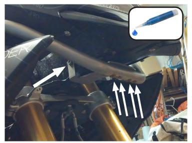
Use 4mm allen wrench, install (4) M6 x 35 flat head screws, attaching bars to center under nose bracket. Apply thread locker to each screw. Tighten to 3 N-m, careful not to strip. Tighten the left and right side 6mm torx screw (T30) on the front bracket to 8 N-m.
