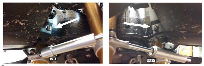
(5) Under the front of the bike, on each side of the headstock of the frame, use T30 Torx and remove the two (2) factory M6 screws as shown.
