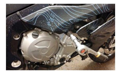
(1) Remove right side engine mount bolt as shown T50 torx tool required. Leave the two spacers in the frame. You will not re-use the bolt.
