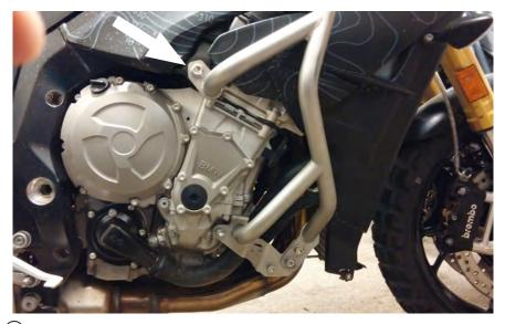
Attach right side bars to bike. Start by sliding the bars together under the nose.
