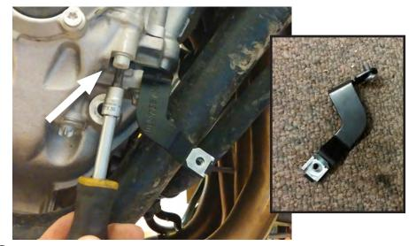
(4) Remove the right side bracket that holds the fairing, use T30 torx. You will not reuse these parts.
