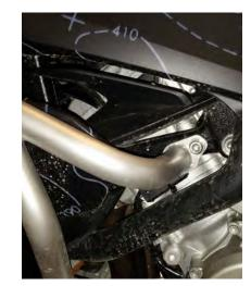
Tighten M8 left side frame mount bolt to 15 N-m.
