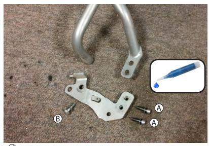
Arrange right side crash bar and right side mounting bracket from bracket kit. Front screws are two M8 x 25 socket cap screws with washers, (A). Rear is M8 x 30 hex cap with washer(B).
