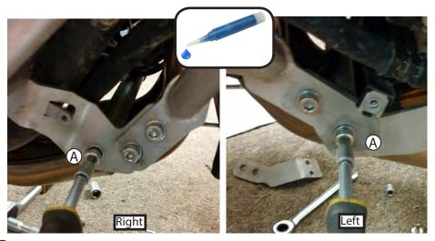
(5) Install low bracket cross tube as shown. Apply thread locker to each screw. Each side uses one M8 x 35 socket cap screw. (A) Attach Loosely for now. **If you are also installing the AltRider Skid Plate**, first remove the M8 screws, and stack the skid plate front brackets on the outside of the crash bar flanges (see pics step 16). Reinstall all hardware.
