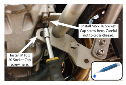
First install M6 screw with washer through lower bracket. Tighten to 5 N-m. Install M10 x 20 socket cap screw with washer (at location shown by arrow), leave loose for now. Apply thread locker to each screw.
