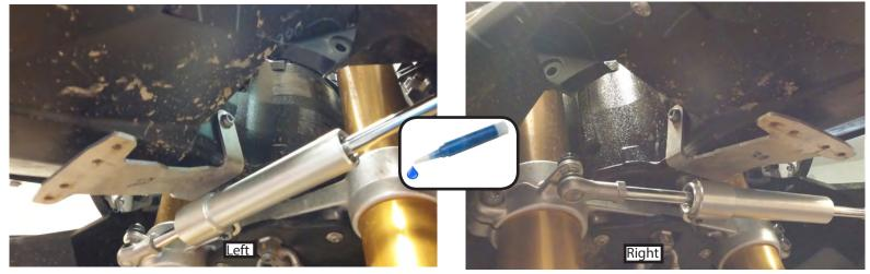
6 Install the front center under-nose bracke. Re-use the factory torx M6 screws. Apply medium strength thread locker to the screws. Do not fully tighten yet.
