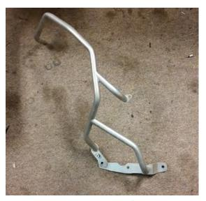
Attach the left side large lower bracket to the left side crash bars as shown. M8 socket head in front position, threaded into permanent nut. M8 hex cap in the rear, going from inside out through bracket and into threaded boss in end of crash bar. Leave screws loose so bracket can be repositioned as needed.
